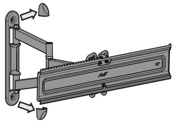
(iii) Adjust nuts to obtain required arm tension.
